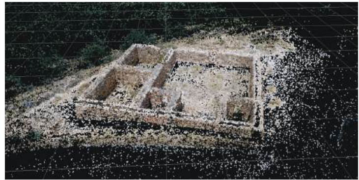
Workflow con Agisoft Metashape: nuvola sparsa
