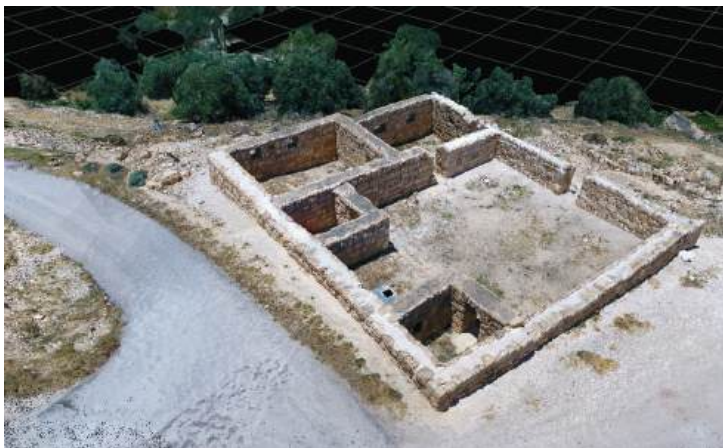
Workflow con Agisoft Metashape: nuvola densa
